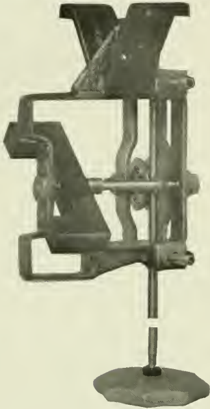
Float and One of the Magnets of the Flow Meter.
